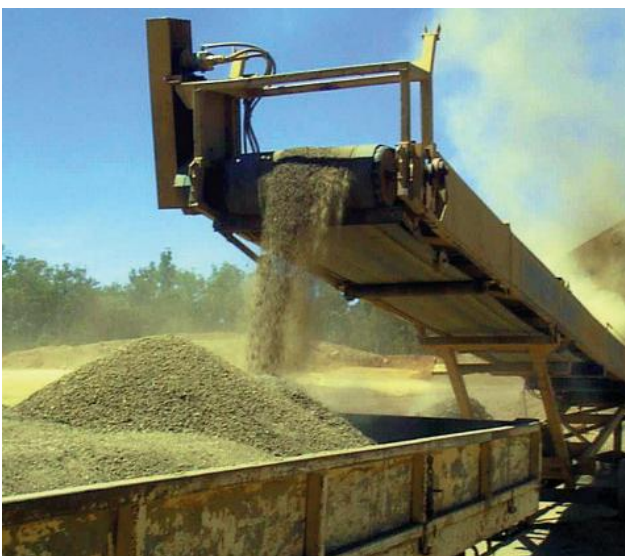
Topsoil is screened to gather a seed-rich mix used to maximise growth in the restored areas (Author: Alcoa World Alumina Australia©)
